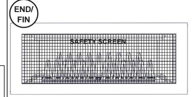
NOTE: CLEANING THE SAFETY SCREEN MAY BE NECESSARY DUE TO EXCESSIVE LINT / DUST FROM CARPETING, PETS, ETC. SIMPLY VACUUM USING THE BRUSH ATTACHMENT.
