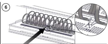
CENTER THE COIL ART OVER THE BURNER PÔRTS. ENSURE THE PILOT OPENING IS TO THE FRONT OF THE APPLIANCE.
