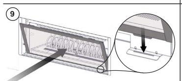
ENSURE THE DOOR IS PLACED INTO THE TWO SLOTS AT THE BOTTOM OF THE APPLIANCE.
