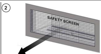
REMOVE THE SURROUND, EQUIPPED WITH THE SAFETY SCREEN. ENLEVER LA FAÇADE, FOURNI AVEC L'ÉCRAN DE PROTECTION.
